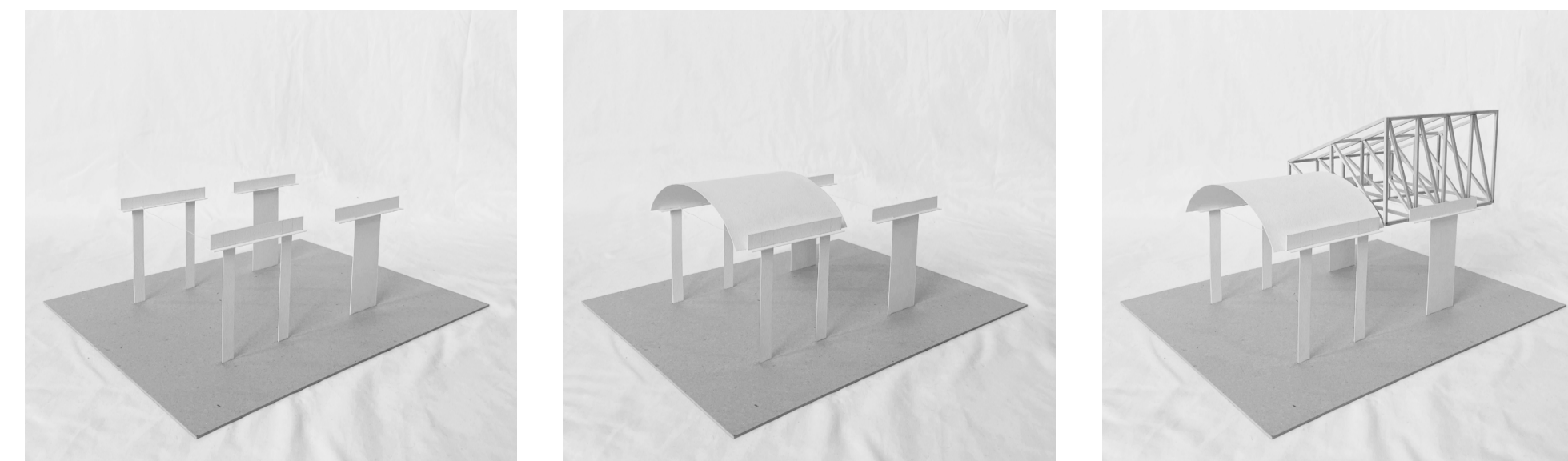
The two types of steel columns will be erected, forming the framework for the space.
