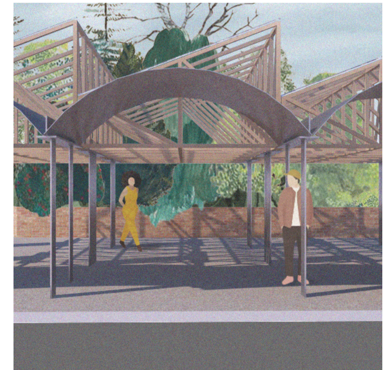
Repeated roof forms reference the sawtooth warehouse roofs but remake these as a series of timber trapezoidal prisms, held aloft to create a space to gather below.
