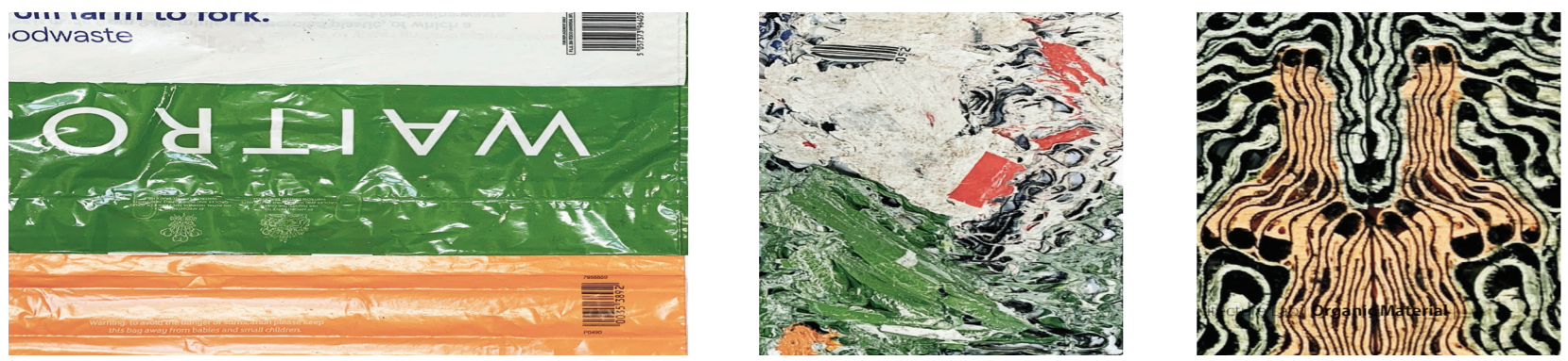
Used plastic shopping bags collected from different supermarkets and offcut fabric rolled together and heated up to 200 degree Celsius in a kiln, heated blocks taken out of the kiln are sliced to reveal the marbled texture
